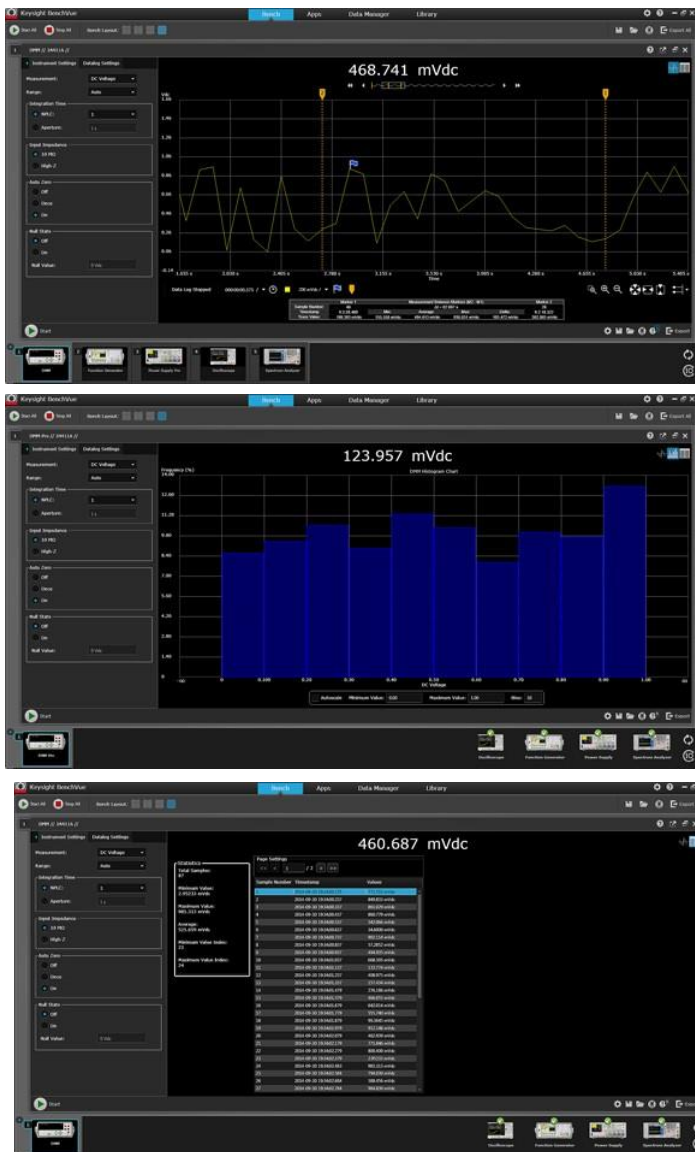
Figure 2. BenchVue enables control of your DMM to data log and visualize measurements in a wide array of display options.
